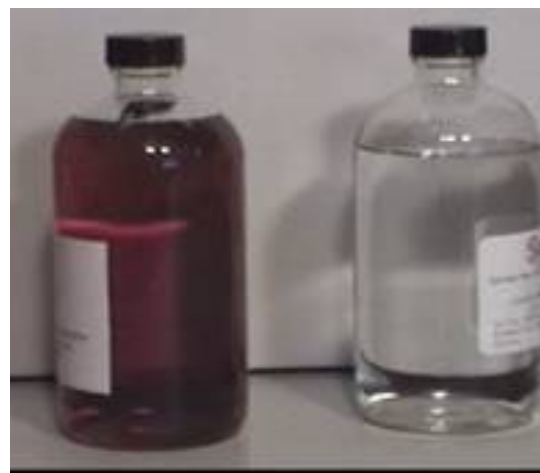
Figure 6.—Synthetic fuel (right) tends to be cleaner than crude-oil-derived Jet-A (left).
